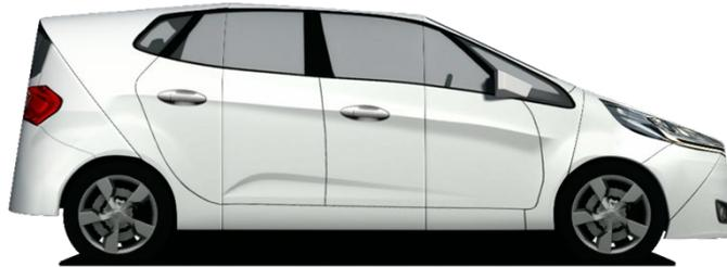
Figure 4-1 Global Vehicle Target (GVT)
