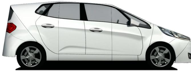
Figure 4-1 Global Vehicle Target (GVT)
